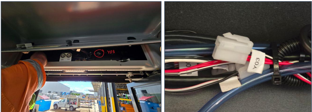
Figure 9 – Connector Y03 behind the front door mechanism cover
