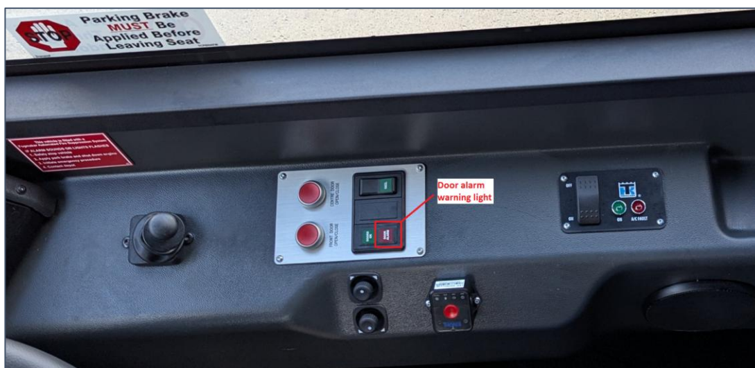
Figure 13 – Door alarm warning light on driver's side console on Optimus
