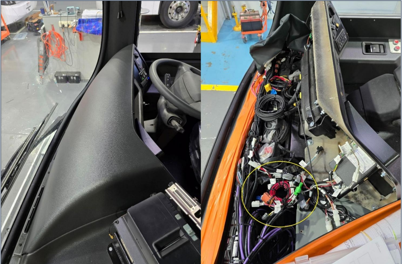
Figure 4 – Dash binnacle cover and location of connector S1305
