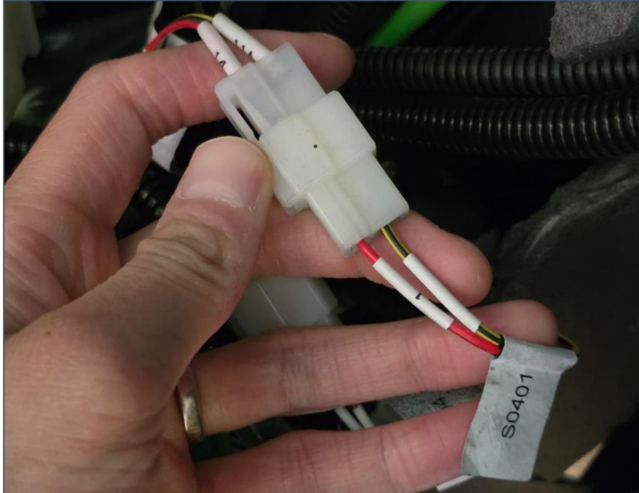
Figure 6 – Connector S0401 above the LHS B-Pillar in the overhead compartment
